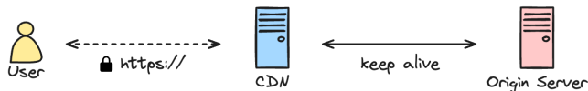
Fig. 6. By terminating the secure connection at the edge, the latency for the user to establish an encrypted connection to the edge server is significantly reduced. The connection to the origin server is kept alive.
